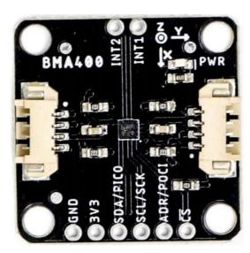
The BMA400 from Bosch Sensortech<sup>©</sup> has a full scale acceleration range of  $\pm 2/\pm 4/\pm 8/\pm 16g$  with exceptionally low current consumption of < 14.5µA while operating at its highest performance settings. The sensor also includes a complete feature set for on-chip interrupts including step counter, activity recognition, orientation detection and tap/double tap.
