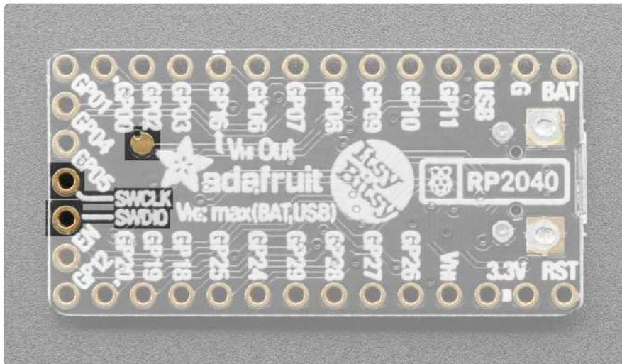
On the short edge of the board are the SWCLK and SWDIO pins. They provide access to the internal Serial Wire Debug multi-drop bus, which provides debug access to both processors, and can be used to download code.
