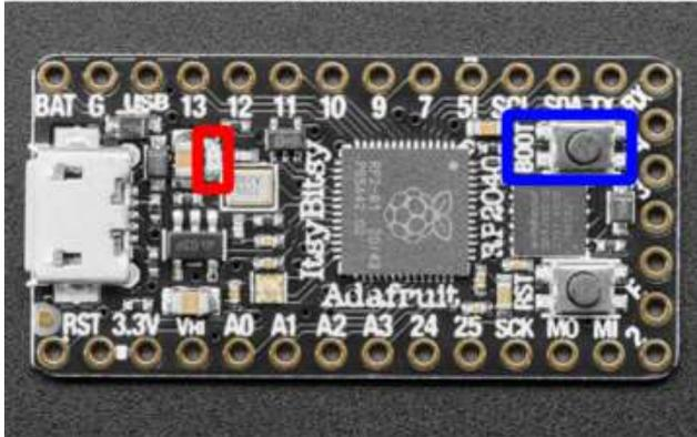
The little red LED (indicated by the red box) is located on the board near the 13 and 12 labels on the silk.
