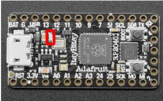
The red LED is located near the 13 on the silk, to the right of the USB connector.
