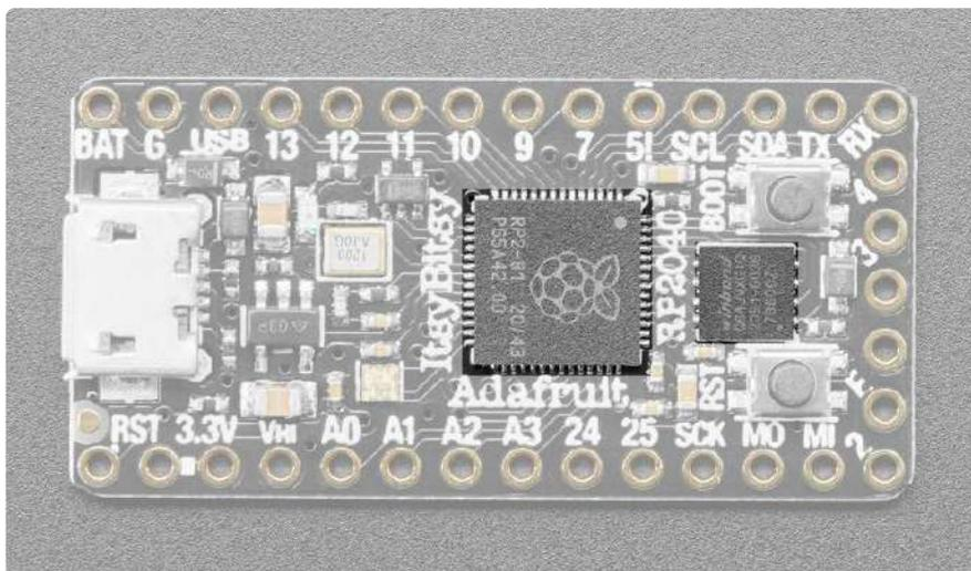
The square towards the middle is the RP2040 microcontroller, the "brains" of the ItsyBitsy RP2040 board.
