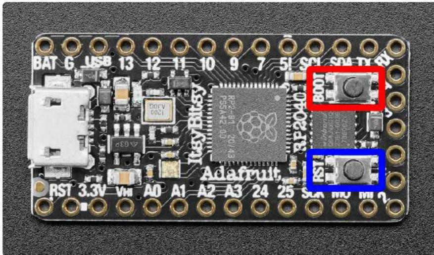
To enter the bootloader, hold down the BOOT/BOOTSEL button (highlighted in red above), and while continuing to hold it (don't let go!), press and release the reset button (highlighted in blue above). Continue to hold the BOOT/BOOTSEL button until the RPI-RP2 drive appears!
