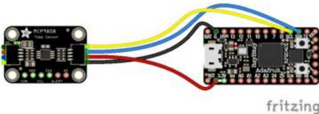
The black wire connects GND on the MCP9808 to ground on your board. The red wire connects VIN on the MCP9808 to power on your board. The yellow wire connects SCL on the MCP9808 to SCL on your board. The blue wire connects SDA on the MCP9808 to SDA on your board.
