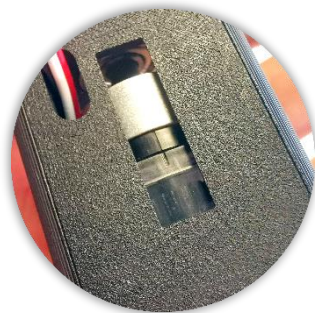
Align the strokes of the motor. Keep the alignment until the end of the process
