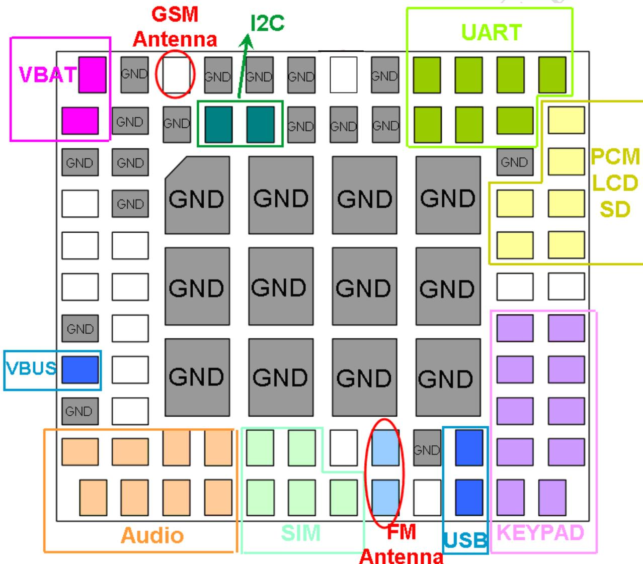
Figure 51: Pin assignment
