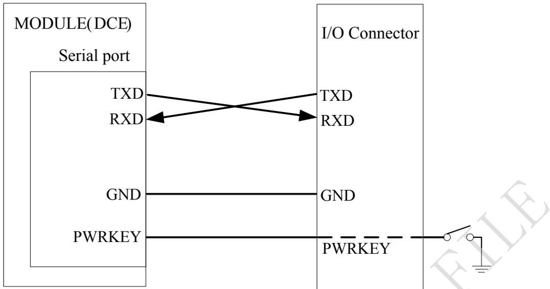
**Figure 25: Connection for software upgrading and debugging**
