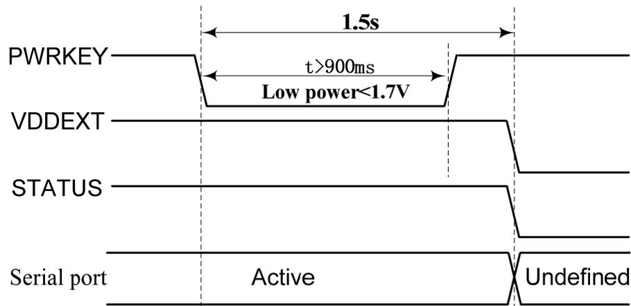
**Figure 13: Timing of power down SIM800L by PWRKEY**
