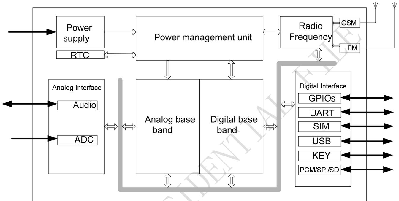
**Figure 1: SIM800L functional diagram**
