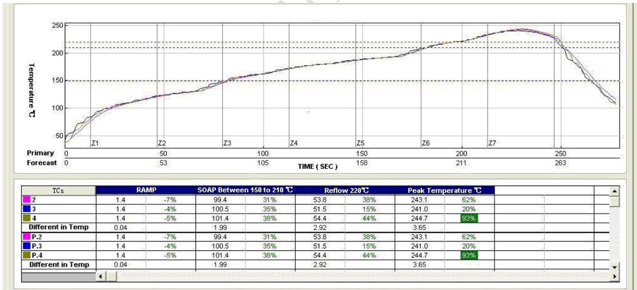
Figure 54: Typical solder reflow profile
