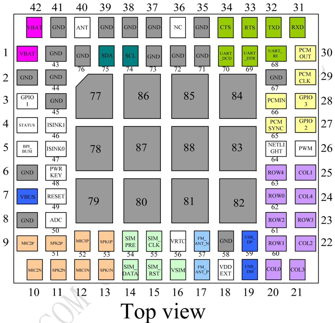
Figure 2: SIM800L pin out diagram (Top view)
