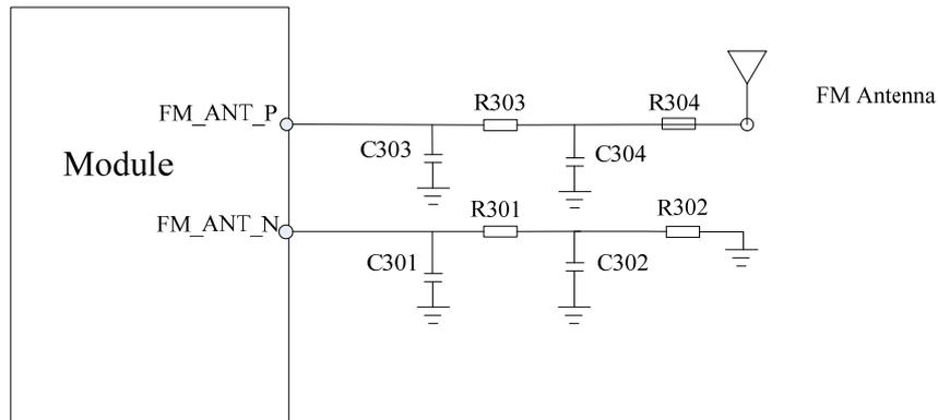
**Figure 49: FM antenna matching circuit**
