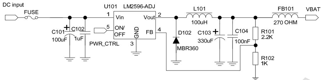
**Figure 7: Reference circuit of the DC-DC power supply**
