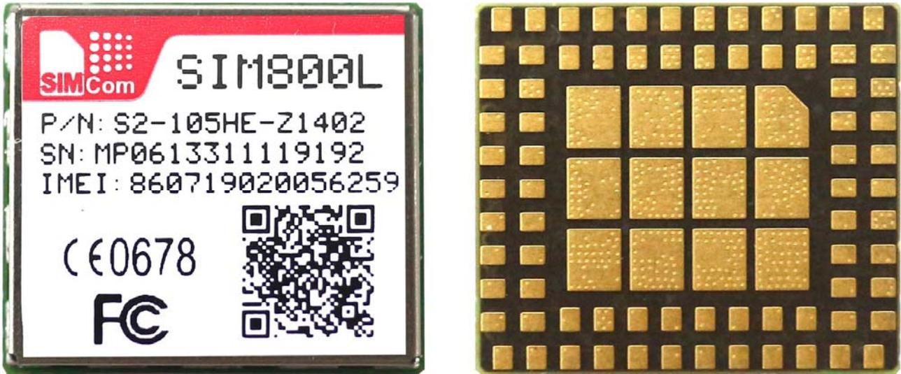
Figure 53: Top and bottom view of SIM800L
