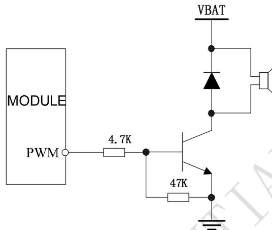
Figure 43: Reference circuit of PWM driver buzzer
