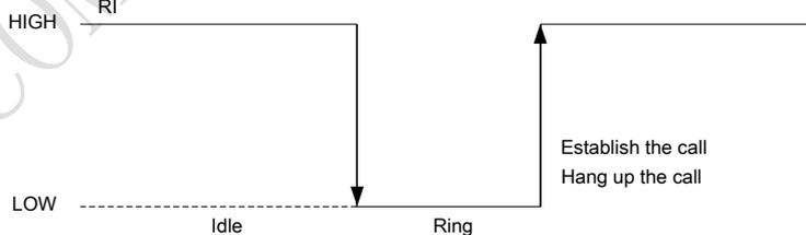
**Figure 27: RI behaviour of data calling as a receiver**
