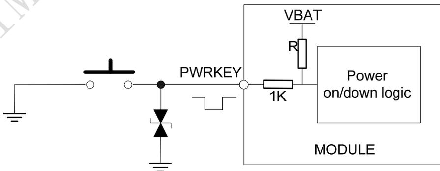
Figure 11: Powered on/down module using button
