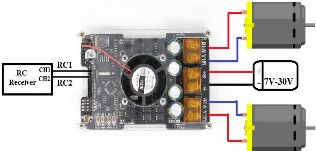
**Sample Connection Diagram of RC receiver and motor with SmartElex 30D.**
