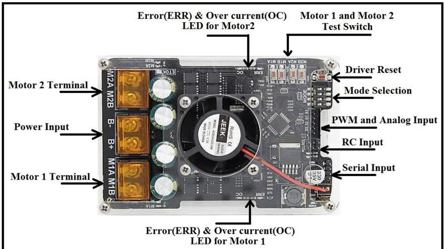
**Power Input:** Connect to a 7V-30V Battery or Power Supply.
