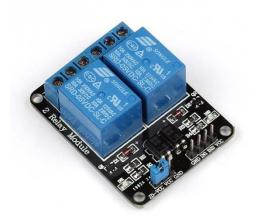
This is a LOW Level 5V 2-channel relay interface board, and each channel needs a 15-20mA driver current. It can be used to control various appliances and equipment with large current. It is equiped with high-current relays that work under AC250V 10A or DC30V 10A. It has a standard interface that can be controlled directly by microcontroller.
