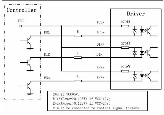
Figure 3: Connections to open-collector signal (common-anode)
