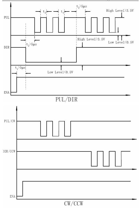
Figure 11: Sequence chart of control signals
