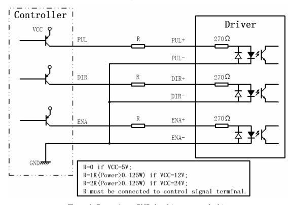
Figure 4: Connection to PNP signal (common-cathode)
