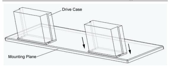
Important NOTE: The driver must be mounted vertically onto a plate or a heat sinking to maximize heat sink area as shown in the above picture. Please use additional heat sinking or cool fan if necessary.
