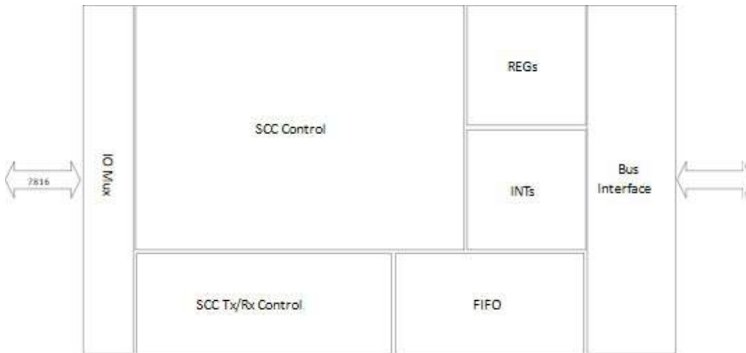
Figure 88. Block Diagram for the Secure Card Module
