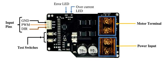
**Power Input**: Connect to a 7V-28V Battery or Power Supply.
