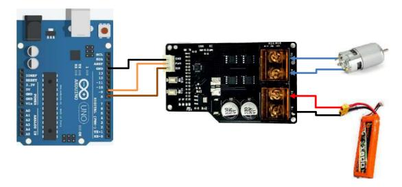
SmartElex 30S can be used with power supplies or batteries. Input power is connected to the power terminals labeled B+ and B-. The input voltage range is 7V to 28V. The input current is dependent on the motors being used and the load placed upon them.
