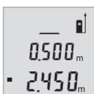
Press the button (6) to add measured values or press the button (3) to subtract measured values. The result will be shown at the bottom of the display after "=", and the current measured value will be shown above it.
