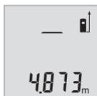
To measure, briefly press the measuring button (2). The measured value will be shown at the bottom of the display.
