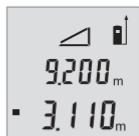
After the second measurement has been completed, the height will be automatically calculated and displayed. The end result will be shown at the bottom of the display, while the current measured value will be shown above it.
