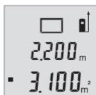
After the second measurement has been completed, the area will be automatically calculated and displayed. The end result will be shown at the bottom of the display, while the current measured value will be shown above it.
