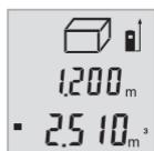
After the third measurement has been completed, the volume will be automatically calculated and displayed. The end result will be shown at the bottom of the display, while the current measured value will be shown above it.
