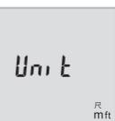
Hold down the on/off button (5). When the required unit of measurement is displayed, release the on/off button (5). After releasing, the measuring tool switches itself on with the selected setting.
