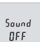
Hold down the measuring button (2) until "Sound OFF" appears on the display (1). After releasing, the measuring tool switches itself on with the selected setting.
