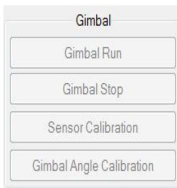
Please calibrate sensors when the output of gyro is far from zero while the gimbal is stationary.
